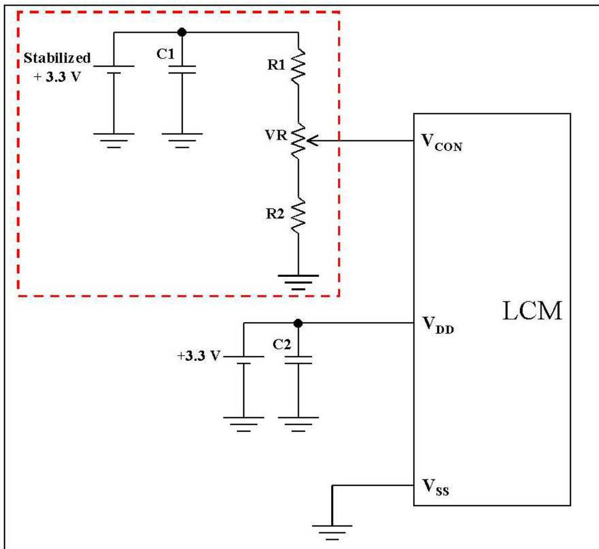
Figure 1: Circuit for modules with build-in DC/DC Converter
