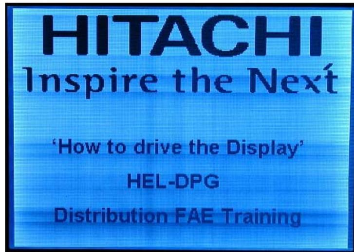
*Figure 5: Result of bad decoupling of a power supply circuit.*
