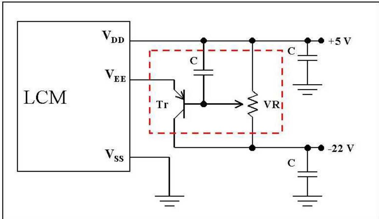
Figure 3: Circuit for modules without DC/DC Converter and Contrast Control Pin
