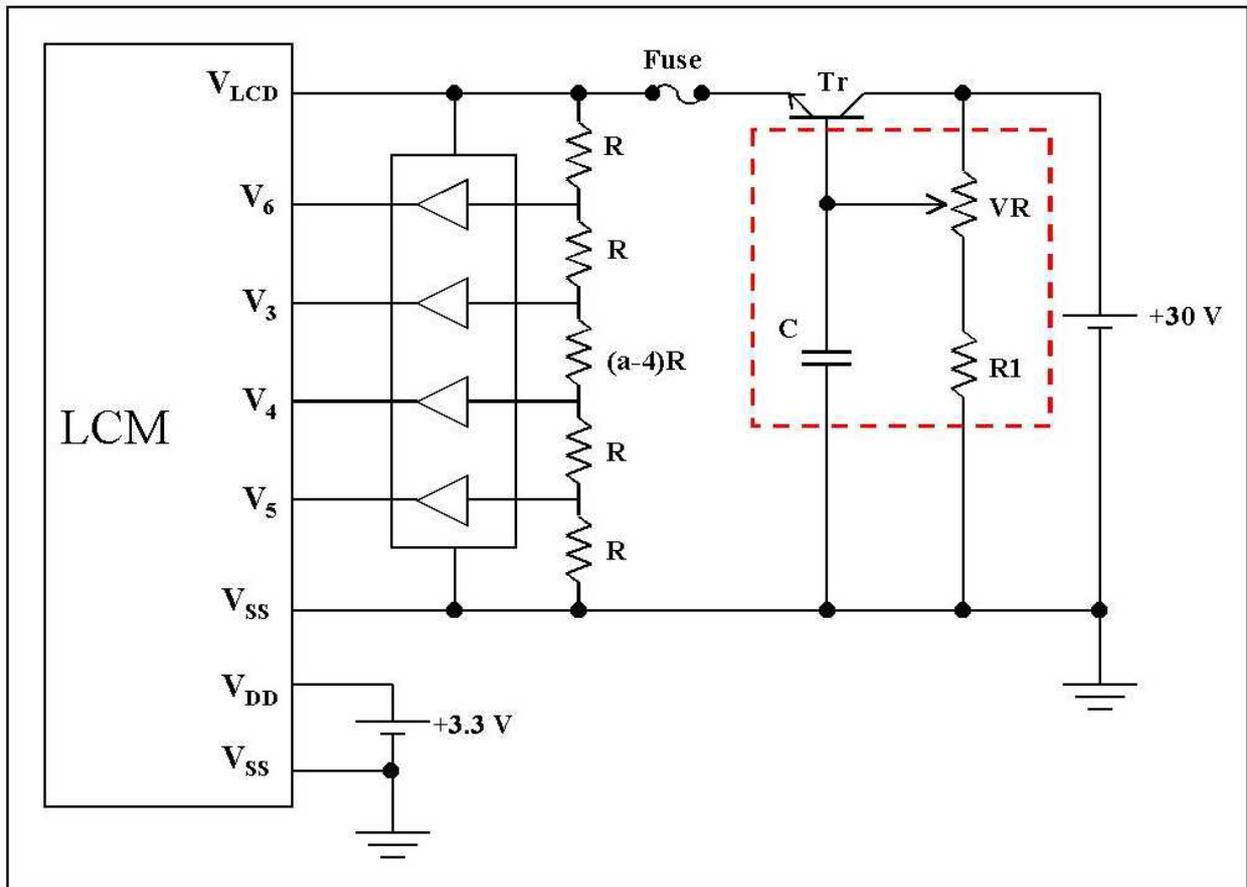
Figure 4: Circuit for modules without any DC/DC circuits on board.
