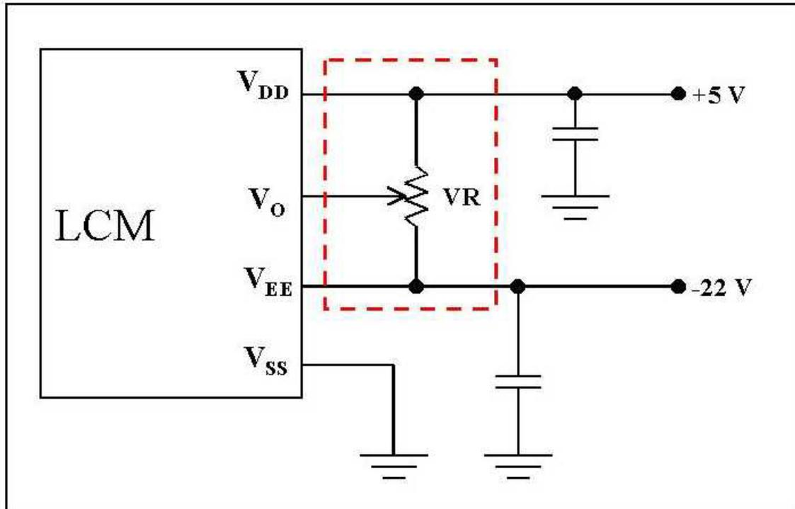
Figure 2: Circuit for modules without build-in DC/DC Converter
